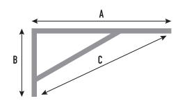
ACB-30: (A)30" (B)16" (C)34" ACB-36: (A)36" (B)16" (C)39" ACB-42: (A)42" (B)16" (C)43" ACB-48: (A)48" (B)16" (C)51"
